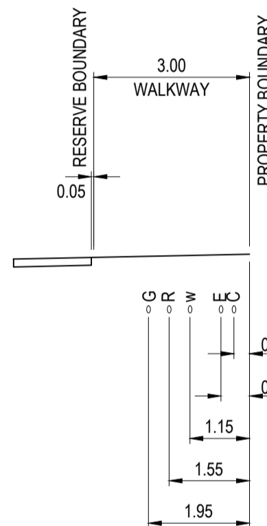
3.0m WALKWAY FYANS WALK TYPICAL SECTION - M
